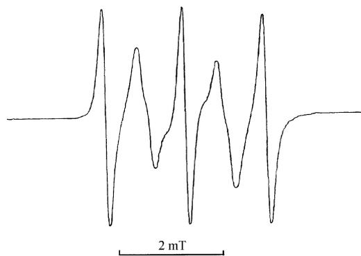
Fig. 3 EPR spectrum of compound **4** in toluene solution ( $c = 1 \times 10^{-4}$  M) at 295 K.
