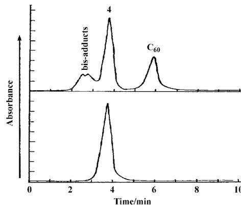
Fig. 1 HPLC data for the reaction mixture (top) and pure compound **4** (bottom). Chromatographic conditions: C<sub>18</sub> reversed-phase column (250 × 4.6 mm, Partisil-5 ODS-3), toluene–MeCN (1 : 1, v/v) as the eluent, UV detection at λ = 328 nm.
