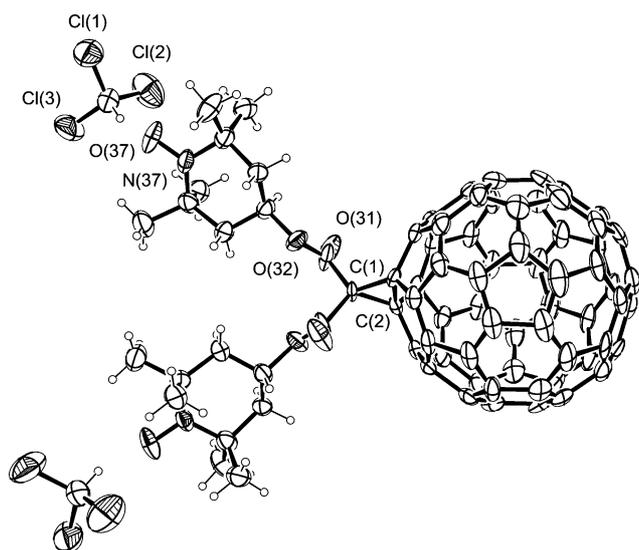
**Fig. 4** ORTEP view of the molecular structure of compound **4**. Displacement ellipsoids are drawn at the 30% probability level. H atoms are represented by circles of arbitrary size. Selected bond lengths and angles are: N(37)–O(37) 1.276(7), N(37)–C(36) 1.486(10), N(37)–C(38) 1.498(11), C(1)–C(2) 1.513(9), O(32)–C(32) 1.218(9), C(1)–C(32) 1.481(9), O(33)–C(32) 1.266(9), O(33)–C(34) 1.467(8) Å; C(2)–C(1)–C(2) 62.5(6)°, C(32)–C(1)–C(2) 120.2(5)°.
